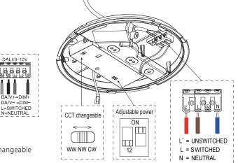
Feed the AC wire into terminal block respectively; If with 3CCT or changeable power function, choose preferred CCT or wattage by slide switch.
